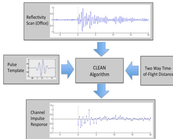
Each P400 UWB transceiver automatically responds to range requests, enabling a single PC connected to one or more transceivers to sequentially query a distributed array of responding transceivers in a floorplan. A real-time demonstration of m multi-node indoor channel assessment with multi-link distance measurement will be presented.
