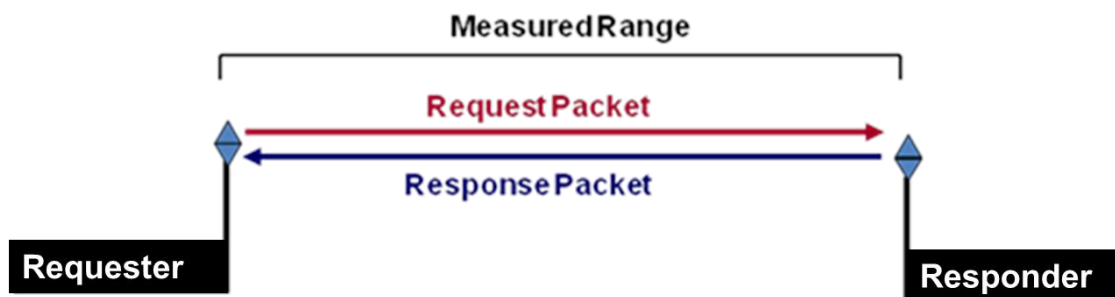
Fig. 1: Packet transmissions required by TW-TOF range measurement
