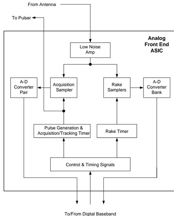
Figure 2. Block diagram of the Analog Front End ASIC.
