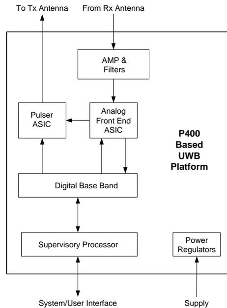
Figure 3. Block diagram of the P400 UWB platform.
