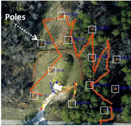
Figure 7. P400 radars (white square) used to track a target (red path) through a terrain (130m x 110m) of mixed forest and meadow.
