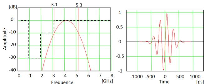
Figure 1. Transmitted waveform in frequency (a) and time domain (b).
