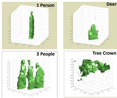
Figure 8. P400 radar images. (from the upper left): person, three people standing close together, the crown of short tree, a deer. All axis span 2 meters. Vertical grid spacing is 0.2m, horizontal grids spacing is 0.5m.
