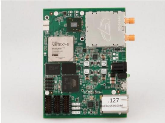
Figure 4. Photograph of the P400 UWB platform (75mm x 100mm).
