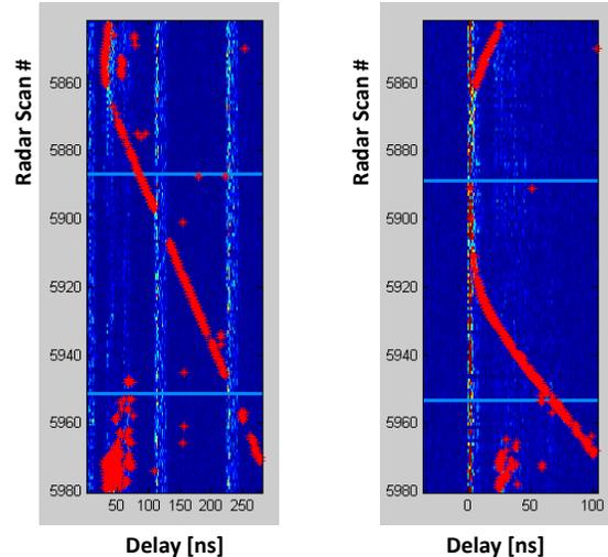
Figure 6. Waterfall plots of mono-static (left) and bi-static (right) radar returns with detection shown in red. Scans rate equal 4 Hz.
