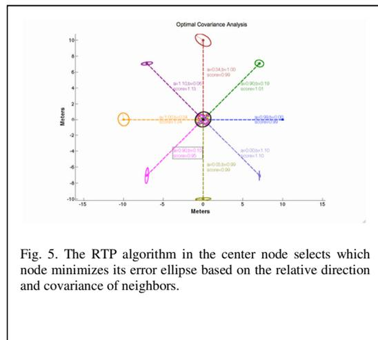
Fig. 5. The RTP algorithm in the center node selects which node minimizes its error ellipse based on the relative direction and covariance of neighbors.
