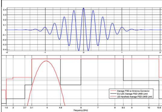
Fig. 2. The time and frequency representation of the basis signal. The signal shape is optimized toward brevity in time while
