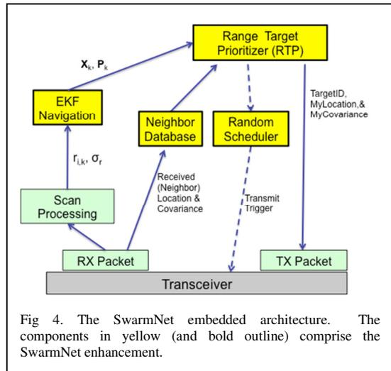
Fig 4. The SwarmNet embedded architecture. The components in yellow (and bold outline) comprise the SwarmNet enhancement.
