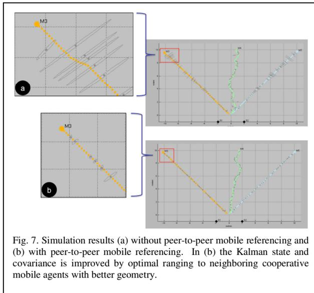
Fig. 7. Simulation results (a) without peer-to-peer mobile referencing and (b) with peer-to-peer mobile referencing. In (b) the Kalman state and covariance is improved by optimal ranging to neighboring cooperative mobile agents with better geometry.
