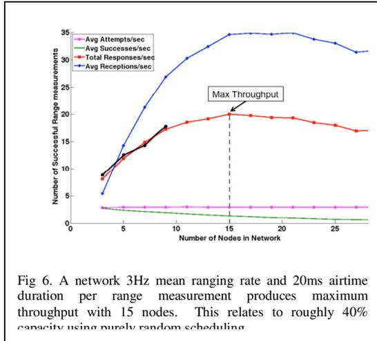
Fig 6. A network 3Hz mean ranging rate and 20ms airtime duration per range measurement produces maximum throughput with 15 nodes. This relates to roughly 40% capacity using purely random scheduling
