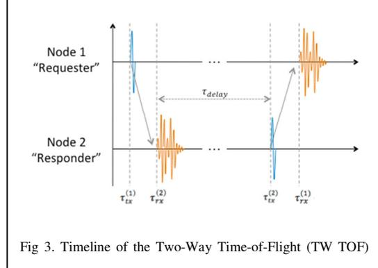
Fig 3. Timeline of the Two-Way Time-of-Flight (TW TOF)
