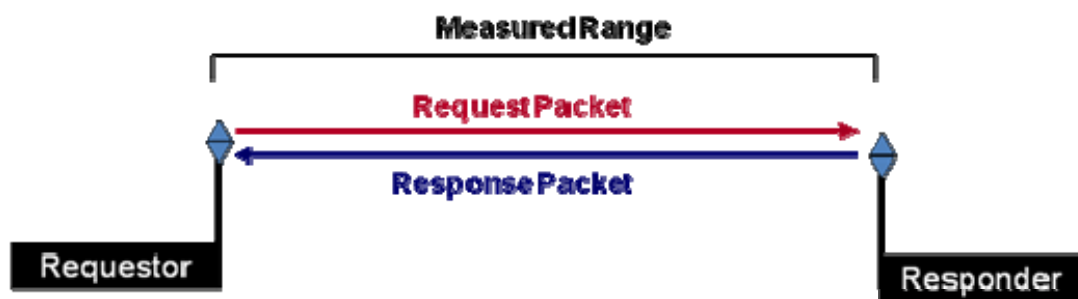
Fig. 7: Packet transmissions required by Two Way Time of Flight range measurement
