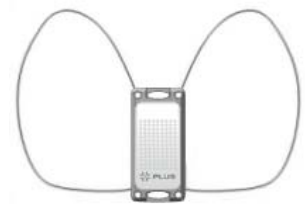
ELEVATION BEAM PATTERN
