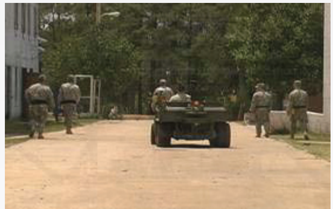
Dismounted soldiers wearing UWB mobile nodes shown being followed by an autonomous vehicle outfitted with UWB coordinate nodes.
