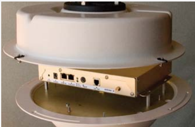
PLUS Reader mounts inside the SFF Antenna
