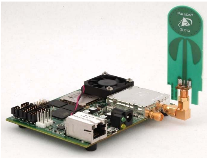
Fig. 1: P400 RCM with attached Broadspec antenna
