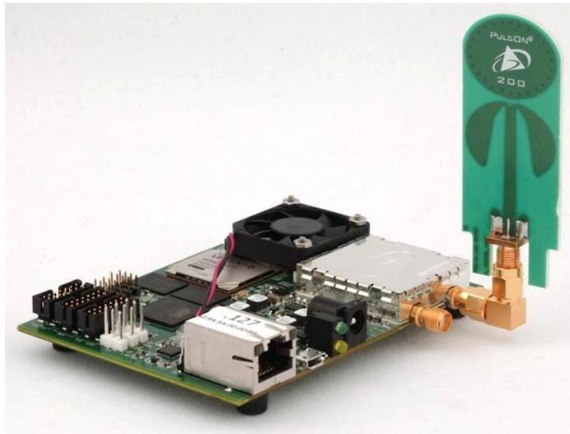
Fig. 1: P400 RCM with attached BroadSpec Antenna
